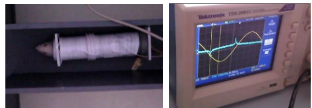
Fig. 4. When the rat enters the pick-up system (left), sharp maxima appear on the pick-up coil (right)
