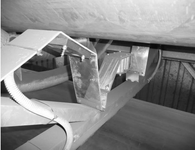
Fig. 2. Sensor placed under the belt
