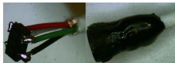
Fig. 3. Final construction: Hall sensor soldered to Vishay cable and protected by Stycast 2850FT epoxy
