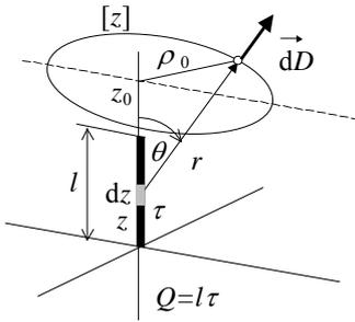
$$dD(\rho_0, z_0) = \frac{dQ}{4\pi r^2}, \quad dD_z = dD \cos \theta, \quad dD_\rho = dD \sin \theta$$
