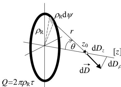
$$dD(z_0) = \frac{dQ}{4\pi r^2}, \quad dD_z = dD \cos \theta, \quad dD_\rho = dD \sin \theta, \quad D_\rho = 0$$
